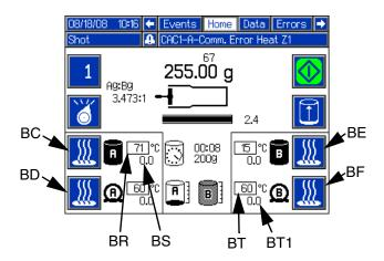
The Tank Fluid Temperature Setpoint (BR), Tank Fluid Temperature (BS), Hose Heater Temperature (BT1), and Hose Heater Temperature Setpoint (BT) display the status of the each of the options. To turn the Tank Blanket Heaters or Hose Heaters on or off, press the Tank or Hose Heater On/Off button (BC, BD, BE, BF). See **Heat Options, Screen #2** on page 28 for more information on temperature control setup.
